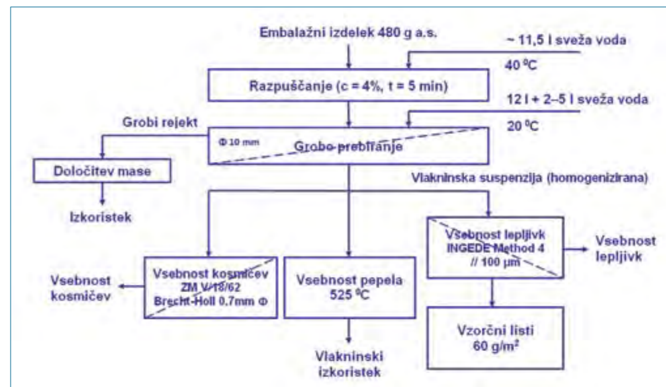
Slika 1. Postopek določanja reciklabilnosti embalažnega produkta – shematski pregled (10) Figure 1. Procedure for packaging recyclability determination – flow chart (10)
