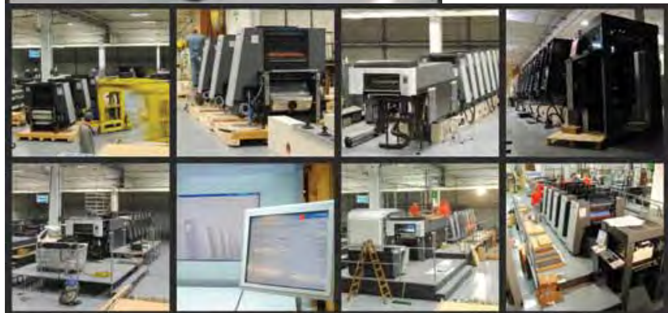
Postopek postavitve stroja Process of installing the new machine
