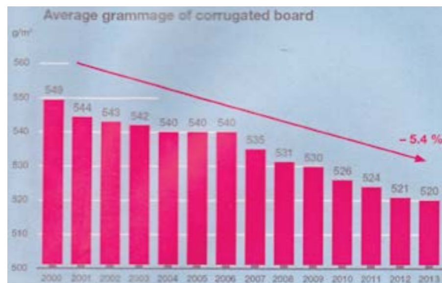
Slika 1: Trend znižanja povprečne gramature valovitega kartona Figure 1: Average grammage reduction rate for corrugated board
